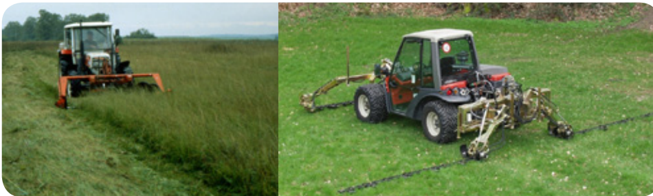
Fig. 3.2.1(4). In comparison, blade mowers are the most gentle mowing machines. This figure shows a modern “butterfly-mowing-machine” (with a front-mower and 2 rear-mowers) with 9m working-width. (Right) and a blade mower which exists for front and rear extension and for working-widths of up to 9m (left).
